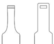
Horizontal Indent T00573 Indent to add root torque.
